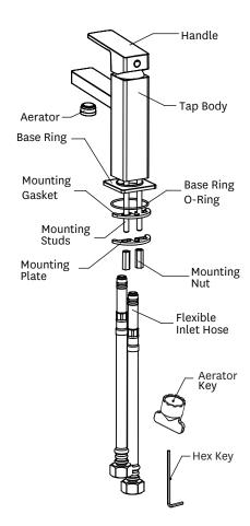
**IMPORTANT:** Before you begin, turn off the water supply. It is recommended to fit isolation valves to both the hot and cold supply.
