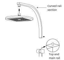
Now take the curved section of the rail and slide this on to the brass fitting on the top end of the main rail section. Position square and central and lock into place using the hex key provided in the grub screw on the back of the main rail section. Take the showerhead ensuring that the rubber washer is in place in the inlet and screw this on to
