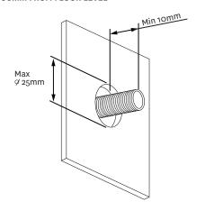
Install a  $\frac{1}{2}$ " male threaded connection at the recommended height on wall, ensuring that a minimum of 10mm of thread protrudes past the finished wall.
