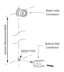
Screw the bottom rail connector to a wall stud or use wall plug making sure it is vertically in line with the top rail connector.
