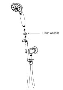
Insert the filter washer into the new hose before screwing to the handset.
