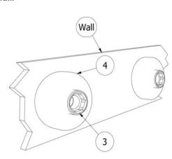
The body (1) may now be offered up to the protruding unions (3) and attached using the appropriate spanner. The mesh filter (2) must be inserted between the join.
