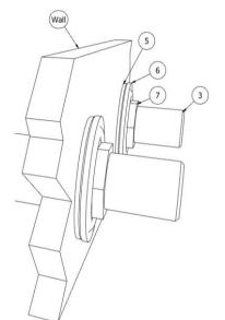
Looking at the wall from the front, the wall shrouds (4) may be screwed over the protruding unions (3) and fixed tight up to the wall.
