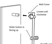
Ensuring the handset slider button is facing upwards as shown in the illustration, adjust the two rail end assemblies to match the position of the wall brackets and turn wall covers anticlockwise to the unlock position. Locking
