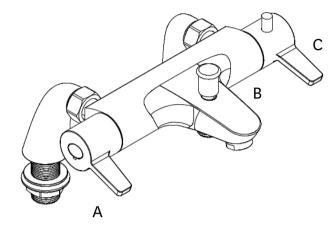
When the diverter (B) is in the lower position, water will flow through the bath filler spout. To divert water through the hose to the shower head, raise the diverter handle to be in the raised position. The diverter will remain raised until manually lowered.
