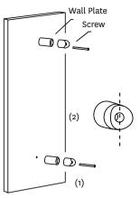
Use a 6mm drill bit to drill a hole in the wall at the desired height, drill a second hole vertically lower at a recommended height of 550mm. In certain situations, the hole may need to be further away to a maximum of 615mm. Place wall plugs into hole and push firmly into place. Place fixing bracket over the wall plugs (1) and insert screw provided, tighten until secure, repeat for second fixing bracket. Push rubber grip into fixing bracket aligning the grove vertically (2)
