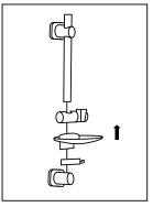
Use a 6mm drill bit to drill a hole in the wall at the desired height, drill a second hole vertically lower at a recommended height of 550mm. In certain situations, the hole may need to be further away to a maximum of 615mm. Place wall plugs into hole and push firmly into place. Place fixing bracket over the wall plugs (1) and insert screw provided, tighten until secure, repeat for second fixing bracket. Push rubber grip into fixing bracket aligning the grove vertically (2)
