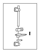
Assemble the handset slider, soap dish and hose retainer on to the rail ensuring button is facing upward (EKITO1/A Lever will face down). Attach both rail end assemblies.
