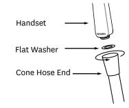
Insert flat washer into the shower hose before screwing to the handset. Connect the other end of the shower to the shower outlet.
