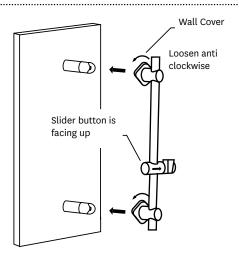
Ensuring the handset slider button is facing upwards (EKITO1/A Lever will face down) as shown in the illustration, adjust the two rail end assemblies to match the position of the wall brackets and turn wall covers anticlockwise to the unlock position.
