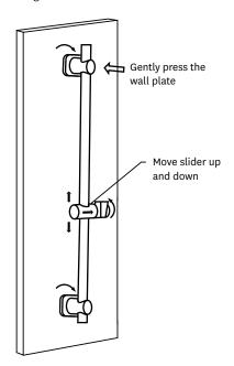
Gently press the rail end assemblies onto the wall brackets, until the rail ends touch the wall. Turn both wall covers clockwise into the locking position, securing the rail. Adjust handset slider to desired height for showing.
