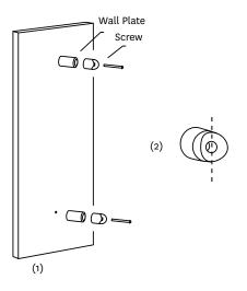
Use a 6mm drill bit to drill a hole in the wall at the desired height, drill a second hole vertically lower at a recommended height of 550mm. In certain situations, the hole may need to be further away to a maximum of 615mm. Place wall plugs into hole and push firmly into place. Place fixing bracket over the wall plugs (1) and insert screw provided, tighten until secure, repeat for second fixing bracket. Push rubber grip into fixing bracket aligning the grove vertically (2)
