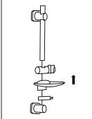
Assemble the handset slider, soap dish and hose retainer on to the rail ensuring button is facing upward. Attach both rail end assemblies.
