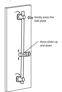
Gently press the rail end assemblies onto the wall brackets, until the rail ends touch the wall. Turn both wall covers clockwise into the locking position, securing the rail. Adjust handset slider to desired height for showing.
