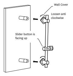
Ensuring the handset slider button is facing upwards as shown in the illustration, adjust the two rail end assemblies to match the position of the wall brackets and turn wall covers anticlockwise to the unlock position.
