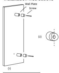
Use a 6mm drill bit to drill a hole in the wall at the desired height, drill a second hole vertically lower at a recommended height of 550mm. In certain situations, the hole may need to be further away to a maximum of 615mm. Place wall plugs into hole and push firmly into place. Place fixing bracket over the wall plugs (1) and insert screw provided, tighten until secure, repeat for second fixing bracket. Push rubber grip into fixing bracket aligning the grove vertically (2)
