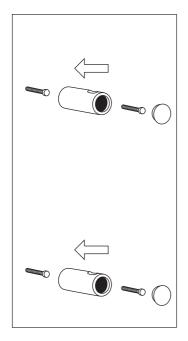
Remove the caps from the end brackets using a sharp blade, taking care not to damage the product.
