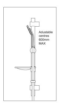
Select location for kit, ensuring no wiring or pipework in the wall can be damaged, also that when the slider bracket is positioned at the top of the rail, the hose is not over extended.
