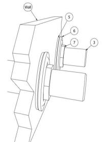
Looking at the wall from the front, the wall shrouds (4) may be screwed over the protruding unions (3) and fixed tight up to the wall.
