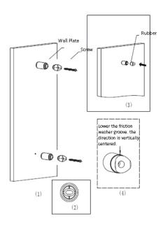
Mount the fixing plate over the hole in the wall as per figure 1, Push the rubber into the fixing plate and place the screw through the rubber and fixing plate into the wall.
