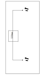
Fit the shower handset into the handset holder of the shower rail kit, place the shower rail kit assembly against the wall to find a suitable place to fix the shower rail kit (Note: when deciding where to fix the shower rail kit, please ensure that the shower hose will not be stretched or subjected to any unnecessary tight bends).
