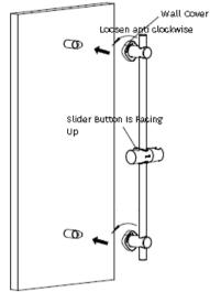
Locking Direction Gently press the wall plate slide Move the Slider up and ()
