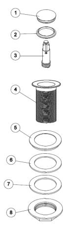
In order to fill the basin, the button in the middle of the waste needs to be pressed down. To release water press the button **to allow drainage**.
