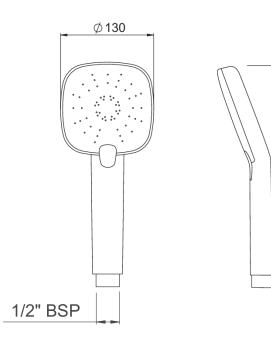
CONSTRUCTION: ABS SUPPLY: Suitable For High Pressure Systems INLET CONNECTIONS: ½" BSP WORKING PRESSURES: 0.5 - 5.0 bar  $\cdot$  Airstream Technology Mixes Air With Water To Create A More Voluminous Spray
