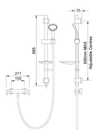
CONSTRUCTION: Brass & ABS SUPPLY: Suitable For High Pressure Systems INLET CONNECTIONS: 15mm Compression WORKING PRESSURES: 1.0 - 5.0 bar CARTRIDGE/VALVE TYPE:Thermostatic
