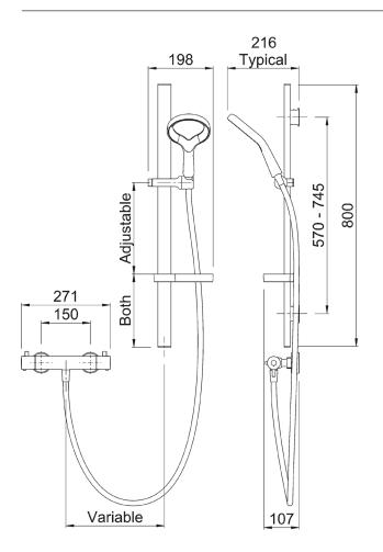
CONSTRUCTION: Brass & ABS SUPPLY: Suitable For High Pressure Systems INLET CONNECTIONS: 15mm Compression WORKING PRESSURES: 1.0 - 5.0 bar CARTRIDGE/VALVE TYPE:Thermostatic
