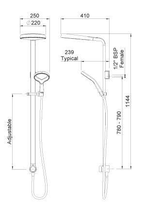
CONSTRUCTION: Brass & ABS CARTRIDGE/VALVE TYPE: N/A SUPPLY: Suitable For High Pressure Systems INLET CONNECTIONS: ½" BSP WORKING PRESSURES: 1.0 - 5.0 bar OPERATION: N/A
