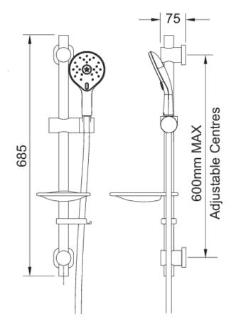
CONSTRUCTION: Brass & ABS SUPPLY: Suitable For All Plumbing Systems INLET CONNECTIONS: ½" BSP WORKING PRESSURES: 0.3 - 5.0 bar CARTRIDGE/VALVE TYPE:N/A
