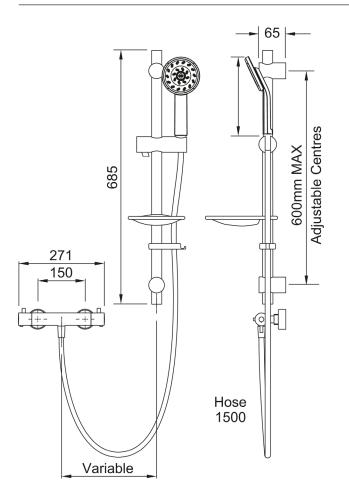
CONSTRUCTION: Brass & ABS SUPPLY: Suitable For High Pressure Systems INLET CONNECTIONS: 15mm Compression WORKING PRESSURES: 0.5 - 5.0 bar CARTRIDGE/VALVE TYPE:Thermostatic
