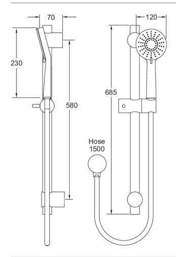
CONSTRUCTION: Stainless steel/ABS SUPPLY: Suitable For All Plumbing Systems INLET CONNECTIONS: ½" BSP WORKING PRESSURES: 0.5 - 5.0 bar CARTRIDGE/VALVE TYPE:N/A
