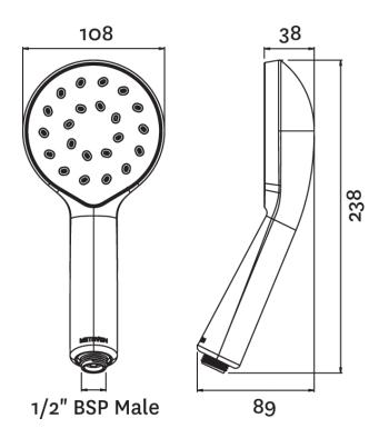
CONSTRUCTION: ABS SUPPLY: Suitable For Low Pressure Systems INLET CONNECTIONS: ½" BSP
