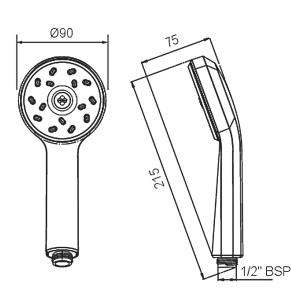
CONSTRUCTION: ABS SUPPLY: Suitable For All Plumbing Systems INLET CONNECTIONS: ½" BSP WORKING PRESSURES: 0.3 - 5.0 bar CARTRIDGE/VALVE TYPE:N/A · Suitable For All Showers
