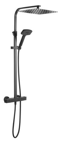
CONSTRUCTION: Brass & ABS Handset CARTRIDGE/VALVE TYPE: Thermostatic SUPPLY: Suitable For High Pressure Systems INLET CONNECTIONS: 15mm Compression WORKING PRESSURES: 1.0 - 5.0 bar OPERATION: Separate Flow And Temperature Controls
