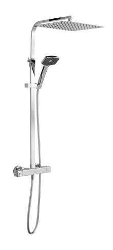
**CONSTRUCTION:** Brass & ABS Handset **CARTRIDGE/VALVE TYPE:** Thermostatic **SUPPLY:** Suitable For High Pressure Systems **INLET CONNECTIONS: 15mm Compression** WORKING PRESSURES: 1.0 - 5.0 bar
