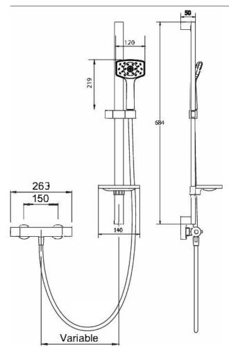
**CONSTRUCTION:** Brass & ABS SUPPLY: Suitable For High Pressure Systems INLET CONNECTIONS: 15mm Compression WORKING PRESSURES: 0.5 - 5.0 bar CARTRIDGE/VALVE TYPE:Thermostatic
