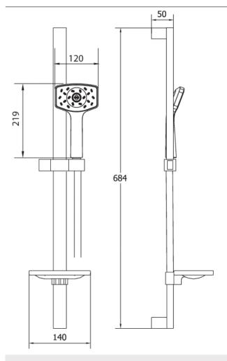
**CONSTRUCTION**: Stainless steel/ABS **SUPPLY**: Suitable For All Plumbing Systems
