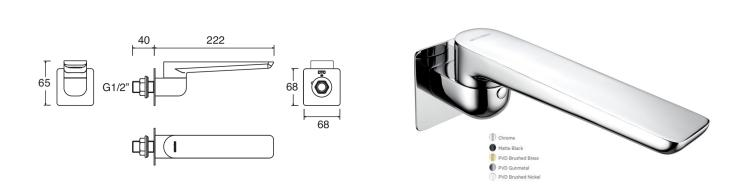
CONSTRUCTION: Brass CARTRIDGE/VALVE TYPE: N/A SUPPLY: Suitable For All Plumbing Systems INLET CONNECTIONS: ½" BSP WORKING PRESSURES: 0.1 - 5.0 BAR OPERATION: N/A
